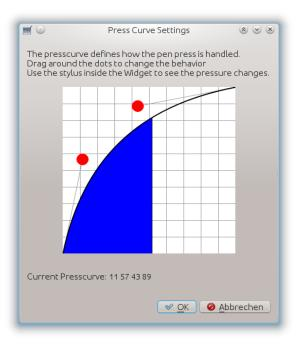
The Presscurve defines how the pressure of the stylus is translated. The Presscurve is defined via four points of a Bézier curve. To change this curve you can alter the red dots and move the curve around.
