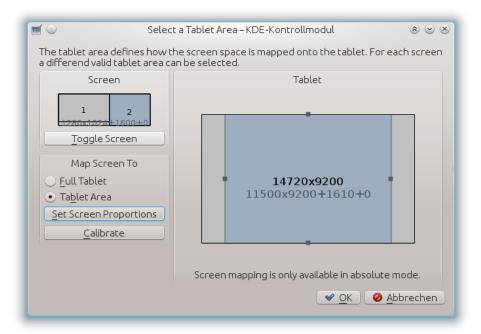
This dialog allows to specify the available tablet area for each selected screen space. In order to keep the aspect ratio of the tablet it is necessary to reduce the tablet area depending on the screen resolution. This Dialog allows to specify them for each screen individually.
